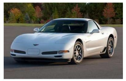
**1997:** Dave Hill makes his mark as the new chief engineer, sweating details to deliver a refined sports car. The 345-hp, LS1 V-8 engine features an aluminum block. A new backbone frame, a rear transaxle, and a small-block moved behind the front suspension add nimble handling to the Corvette's long-standing virtues of high performance and affordable price. Our Csaba
